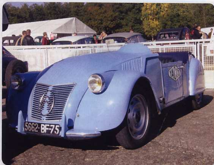
The modified Citroën 2 cv Barbot achieved an average speed of 90.960 km/h for 12 hours at Montlhéry in 1953 with a 348 cc motor.
